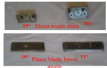
Plate 1 Cutting blades of different angles
